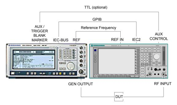
The generator is controlled via the – optional – second GPIB interface of the R&S FSP (= IEC2, supplied together with the option). With some Rohde & Schwarz generators, it is also controlled via the TTL synchronization interface that is contained in the AUX CONTROL interface of the R&S FSP.
