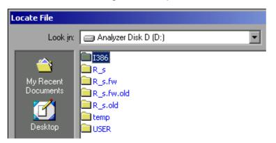
Select the path D:\I386 by turning the rotary knob and then pressing it. If the background of the selection bar is not blue, the selection must be marked with the arrow up/down keys before the entry can be selected by pressing the rotary knob.
