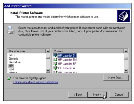
Select the appropriate manufacturer under *Manufacturers* and then the appropriate printer driver under *Printers*.
