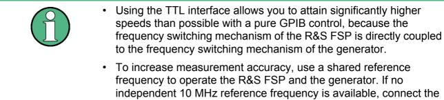
independent 10 MHz reference frequency is available, connect the reference output of the generator to the reference input of the R&S FSP and use SETUP – REFERENCE EXT to configure the R&S FSP to implement the external reference.
