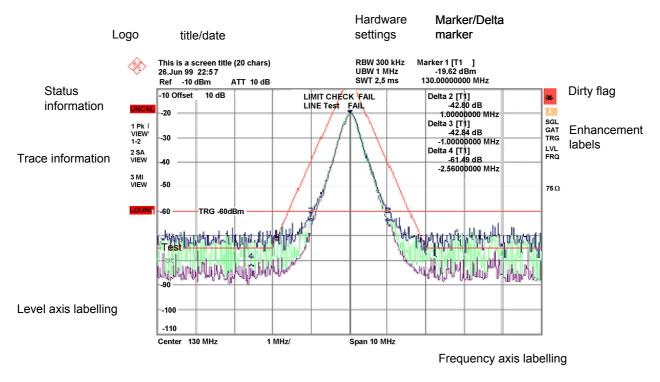
Fig. 4-1 Screen layout of the R&S FSP during analyzer operation
